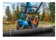
All Genie telehandlers come equipped with a lift shackle that enable you to sling a load without secondary attachments. A factory lift shackle lift chart provides clear capacity limitations to the operator.
