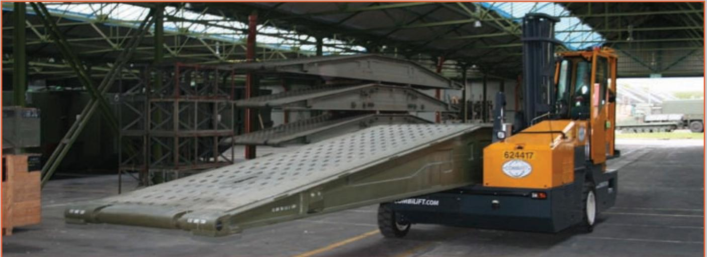
Two C10,00SL Combilifts have been drafted in by the UK Defence Storage and Distribution Agency (DSDA) to work at its vehicle and equipment storage facility due to the extreme maneuverability and versatility they offer for handling a very specific and problematic type of load – components for assembling tank and infantry bridging.
