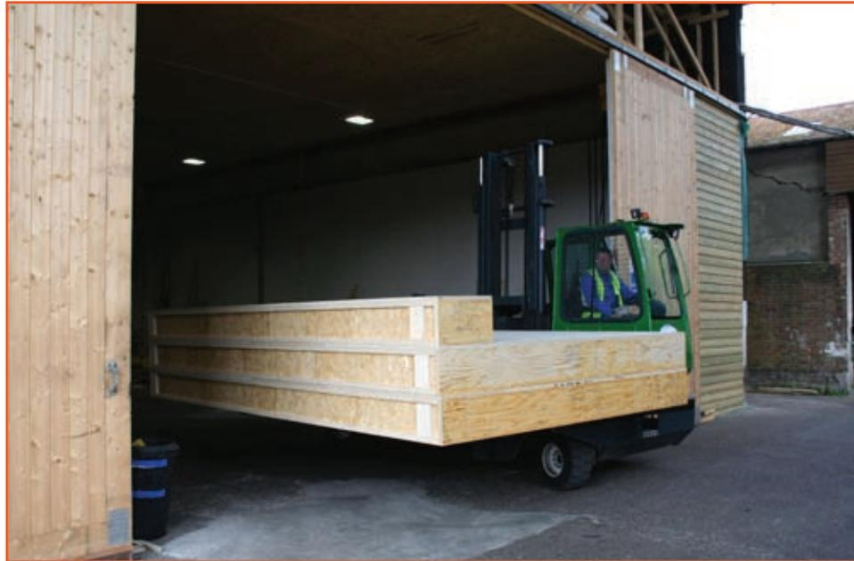
Combilift's sideloaders are tough workhorses for a host of applications. The 4-way models offer the benefits of narrow aisles, great manoeuvrability and the ability to block or bulk stack. The 4-wheeled, two directional sideloader was developed for operations that require reliable, robust and fast operation when moving product across extensive sites and offers considerable benefits over other machines on the market.
