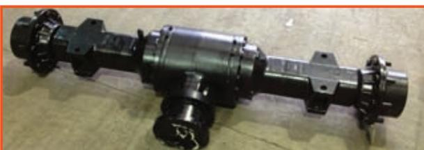
Single hydrostatic drive motor coupled to a JCB differential axle ensures reliable continuous drive for long distance travel
