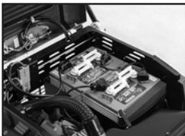
Hood opens providing full maintenance and service accessibility to the battery compartment.
