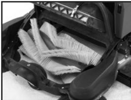
Time-saving maintenance: Broom replacement, and other routine maintenance, can be performed without tools.
