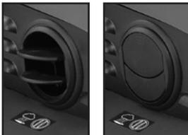
Wet sweep bypass protects the filter from water fouling when sweeping in wet conditions.
