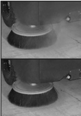
DustGuard™ suppresses side broom generated dust allowing continuous use, and increasing, dust controlled productivity by over 70%.
