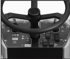
The SW4000™ offers One-Touch™ sweeping with a single switch. Integration with the drive pedal ensures and minimizes broom wear and maximizes run-time.
