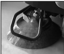
The optional DustGuard™ misting system provides up to 75% greater dust controlled sweeping path for superior indoor air quality and maximizes sweeping efficiency.
