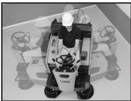
Front-wheel powered and steered drive wheel provides superior maneuverability, allowing operators to sweep in tight corners or narrow aisles.
