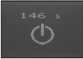
Customizable timeout countdown shuts the machine off after 5 minutes of inactivity for enhanced safety and efficiency.
