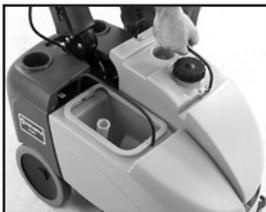
Easily remove the recovery and solution tanks to fill, drain and clean them away from the machine.
