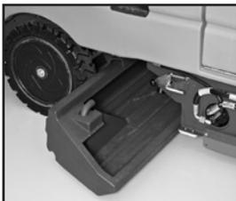
Corrosion resistant hopper slides out easily for maintenance.
