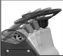
Clear-View™ design and adjustable tilt steering column enable an ergonomic ride for most operators.
