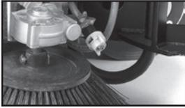
Side broom when equipped with DustGuard™ minimizes fugitive dust generation and provides optimal sweeping performance. (optional)
