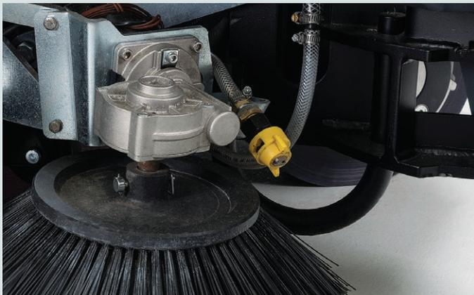
DustGuard™ minimizes side broom fugitive dust generation and provides optimal sweeping performance. (optional)
