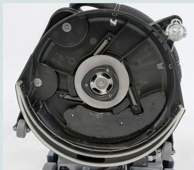
The SC351™ squeegee system provides increased vacuum performance for better water pick-up. The tools-free squeegee can be easily and comfortably removed for cleaning.
