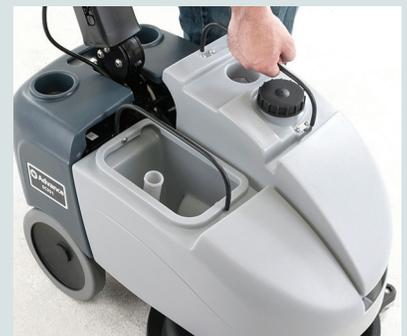
Easily remove the recovery and solution tanks to fill, drain and clean them away from the machine.
