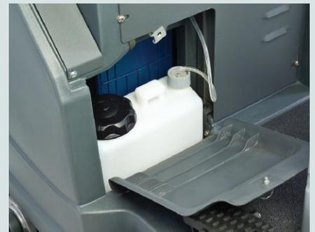
Easy access to onboard detergent dispensing system bottle on EcoFlex™ System.
